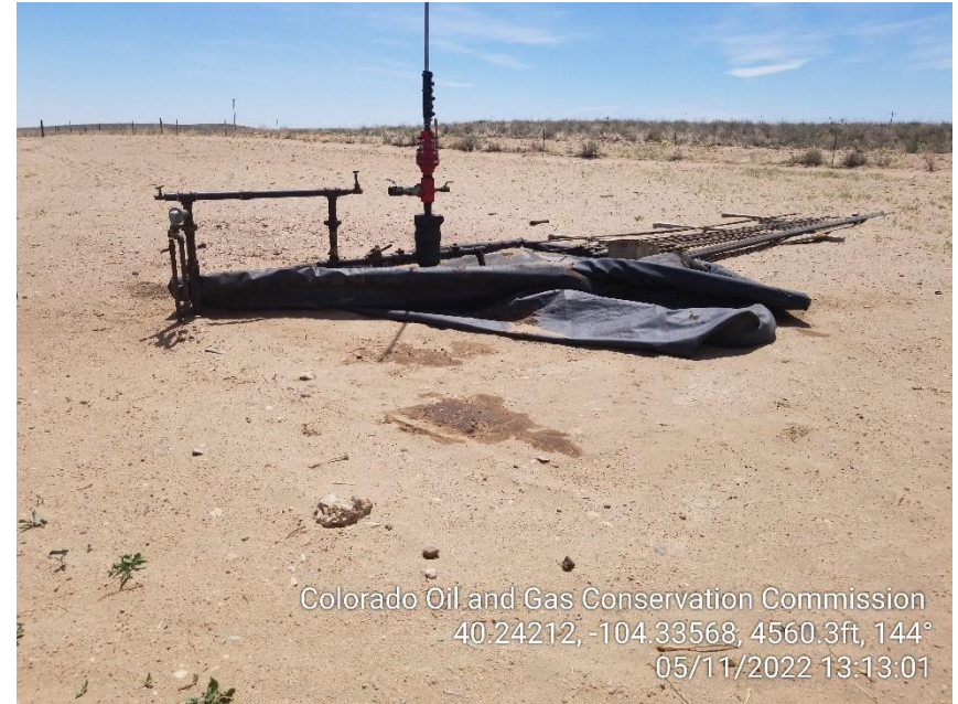
Photo 2 – Wellhead – Unused Rods and Stained Soil
