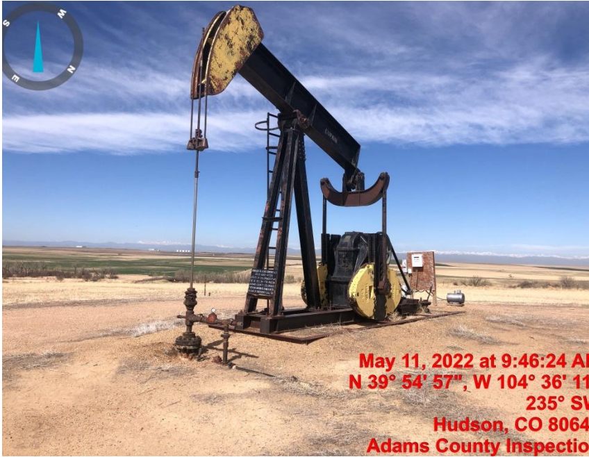
Photo#9 Pumpjack & Wellhead
