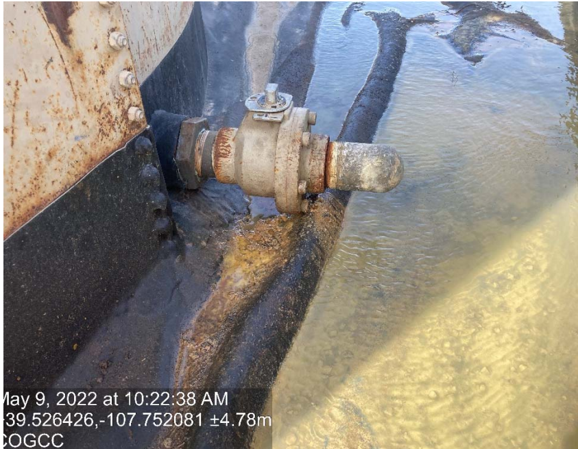
Valve on tank actively leaking
