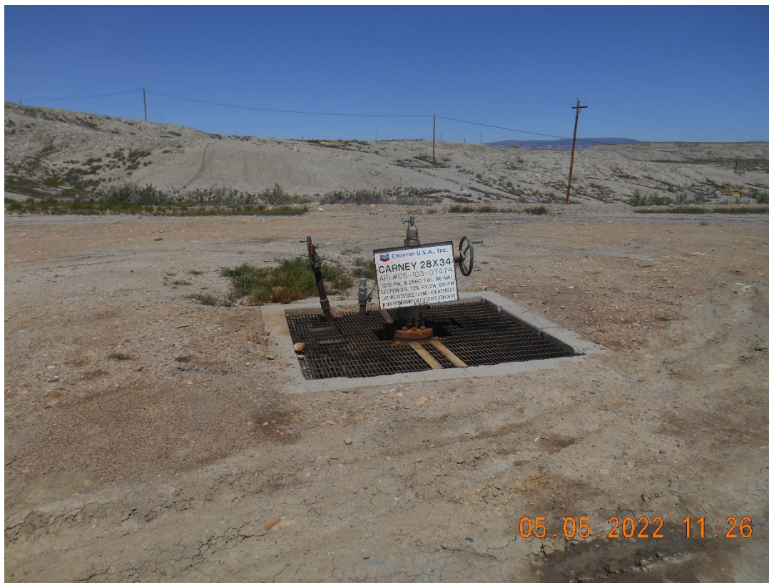
Injection wellhead – Temporarily abandoned
