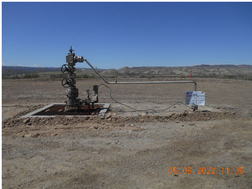
Injection wellhead
