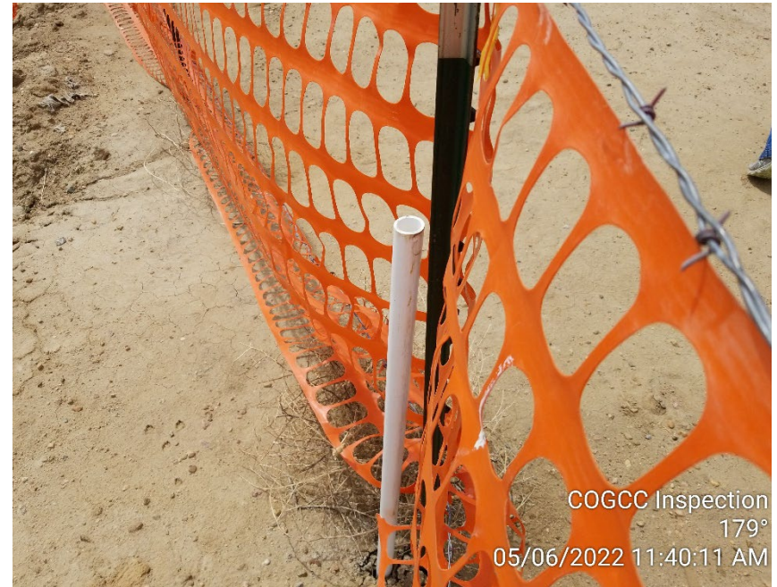
Photo 8 – Uncapped monitoring well.
