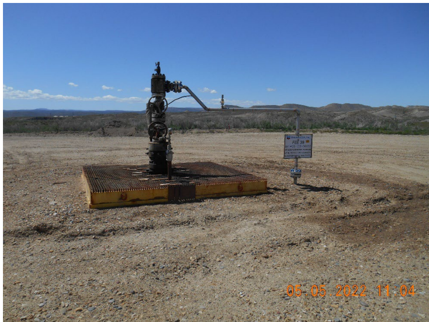
Injection wellhead
