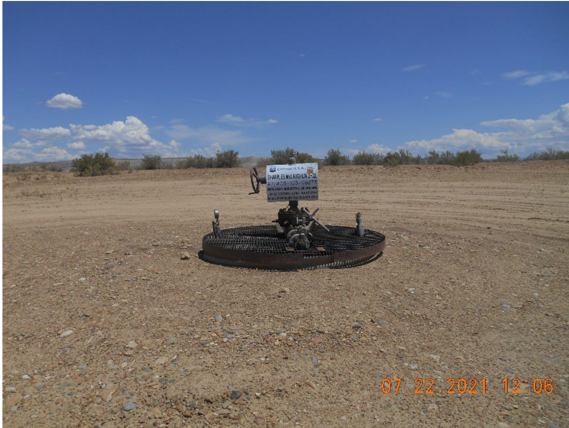
Injection wellhead. Temporarily Abandoned.
