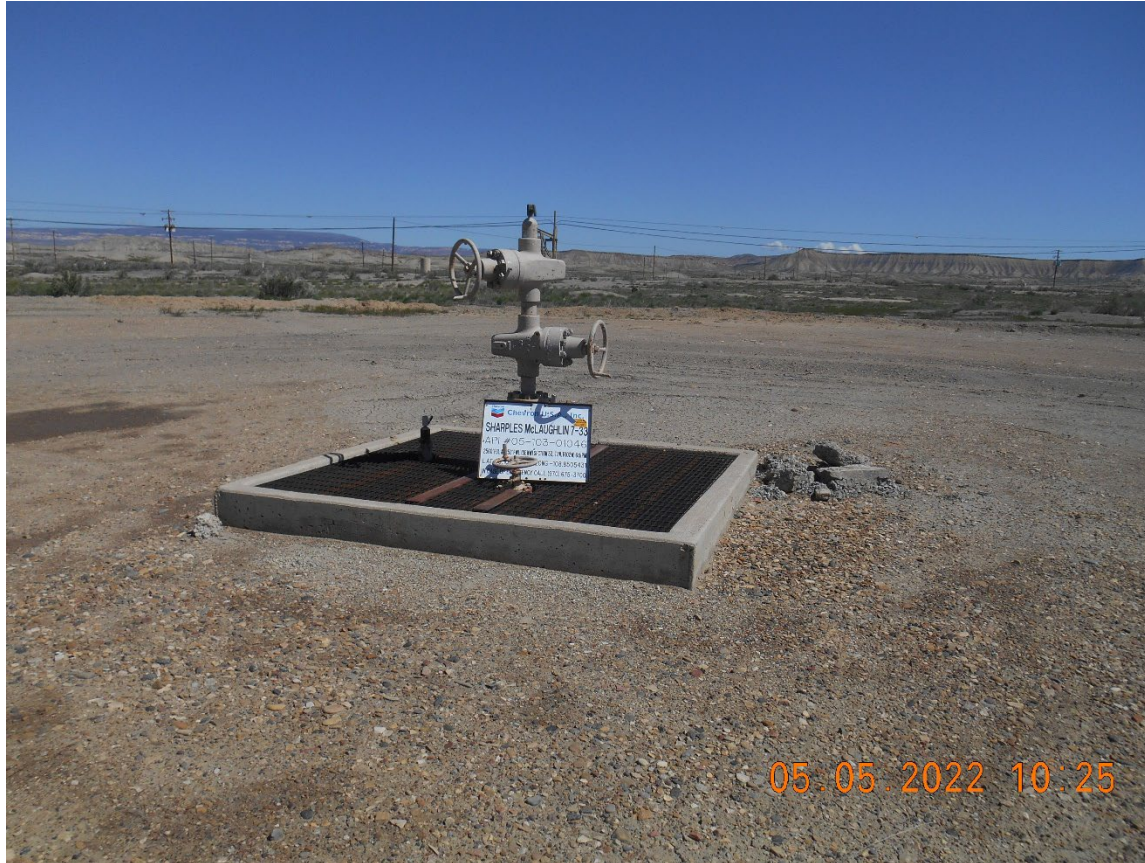
Injection wellhead . Temporarily abandoned
