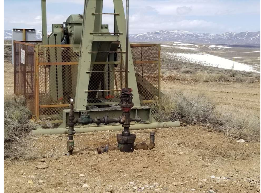
Photo 2. No bradenhead access apparent.
