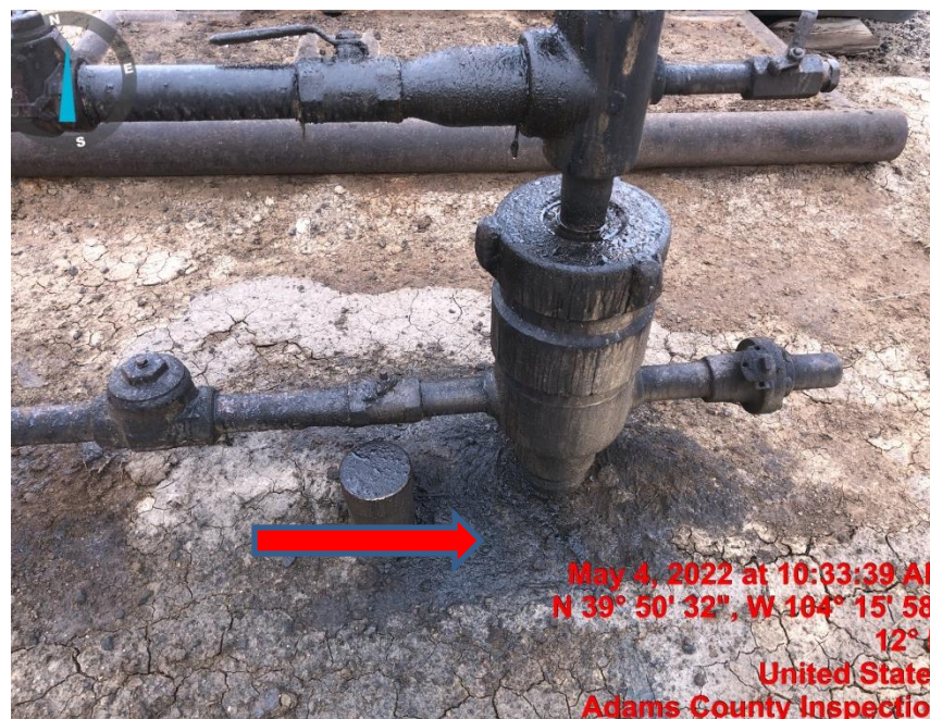
Photo#4 Stuffing box leaking causing stained soil
