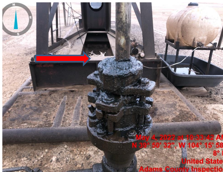
Photo#3 Stuffing box leaking causing stained soil
