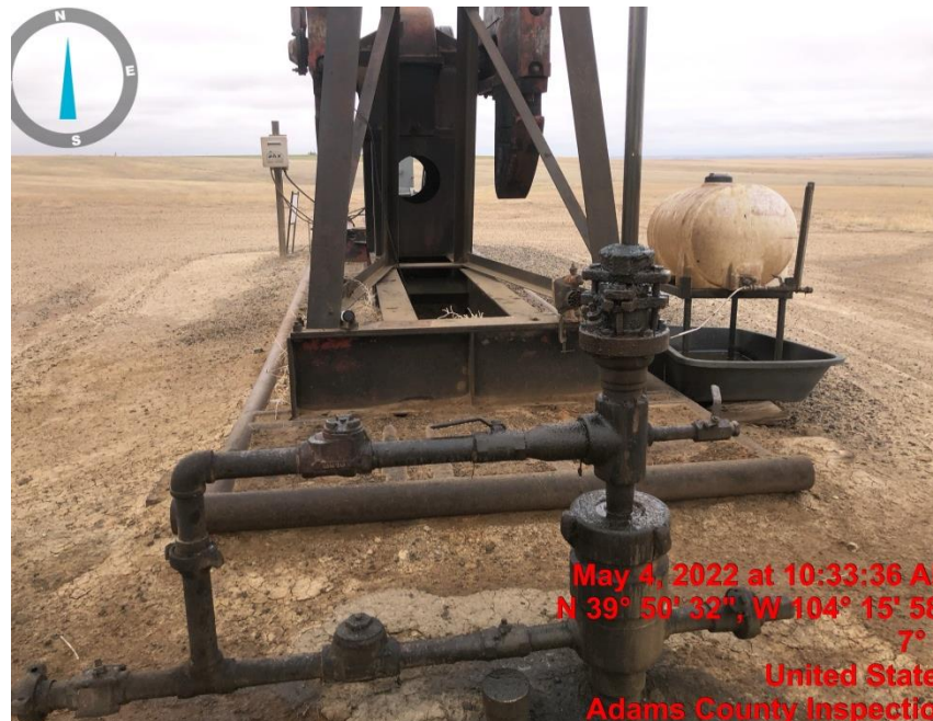
Photo#2 Stuffing box leaking causing stained soil
