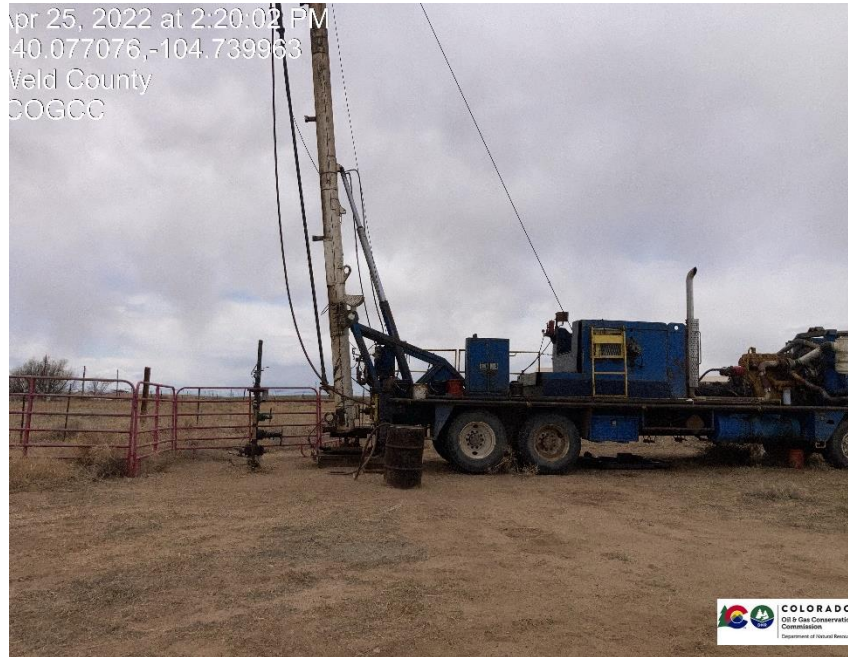
Pic 1 wellhead, swab rig, no crew on site at time of inspection.
