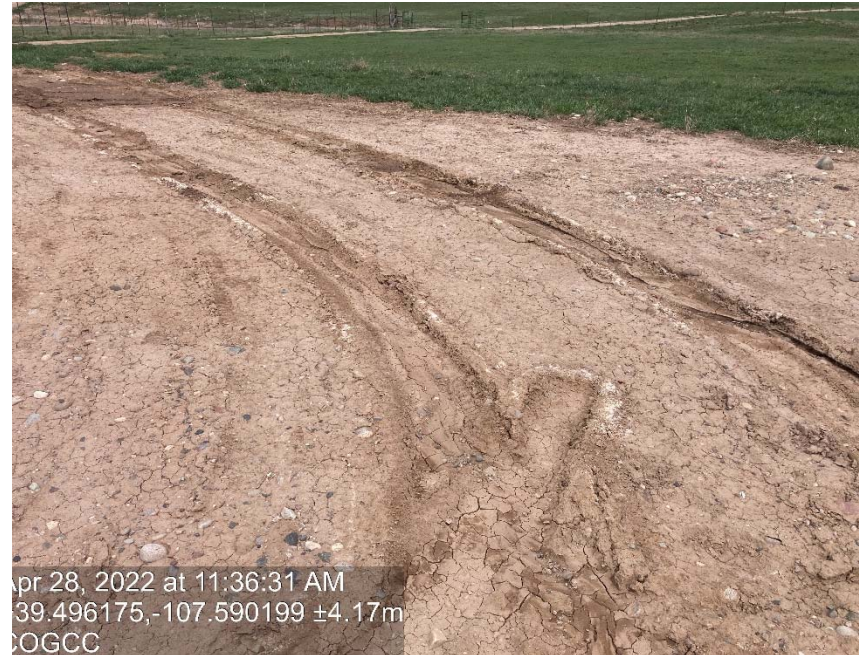
Lack of stabilization/compaction and evidence of irrigation run on
