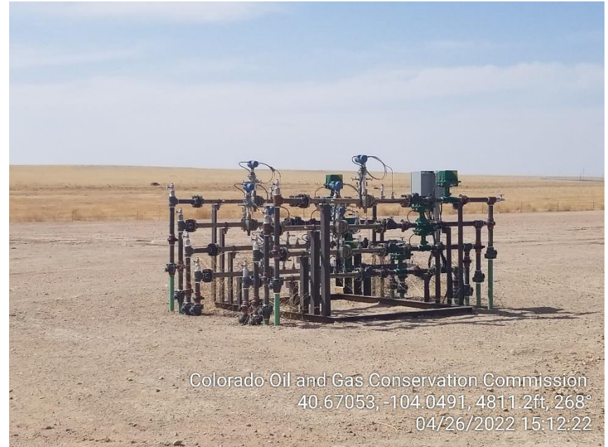
Photo 4 – Gas Lift Injection Meters
