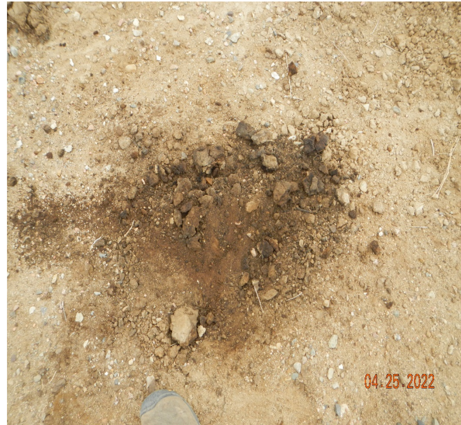
Photo 16. There was oily soils found at center of the location which needs to be cleaned up.
