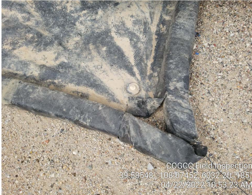
Photo #5 - Mobile separator secondary containment device in need of repair.
