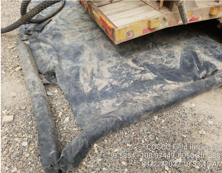
Photo #7 - Mobile separator secondary containment device in need of repair.
