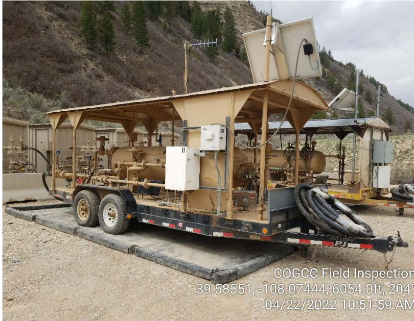
Photo #3 – Mobile separator units located in southwest corner of pad.
