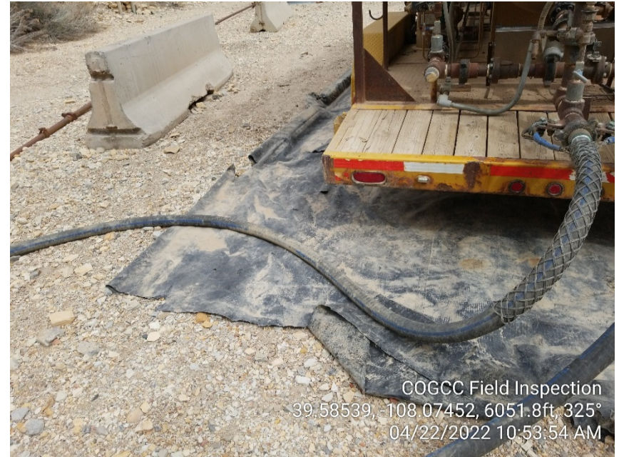
Photo #8 - Mobile separator secondary containment device in need of repair.
