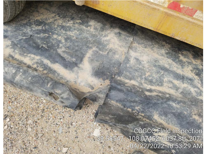
Photo #6 - Mobile separator secondary containment device in need of repair.
