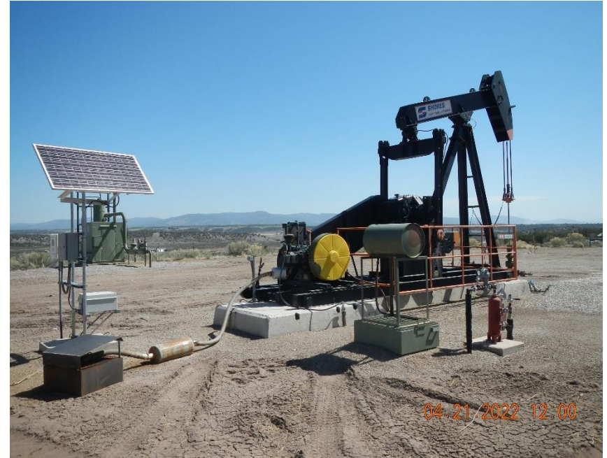
Secondary containment for lube oil container and exhaust outlet.
