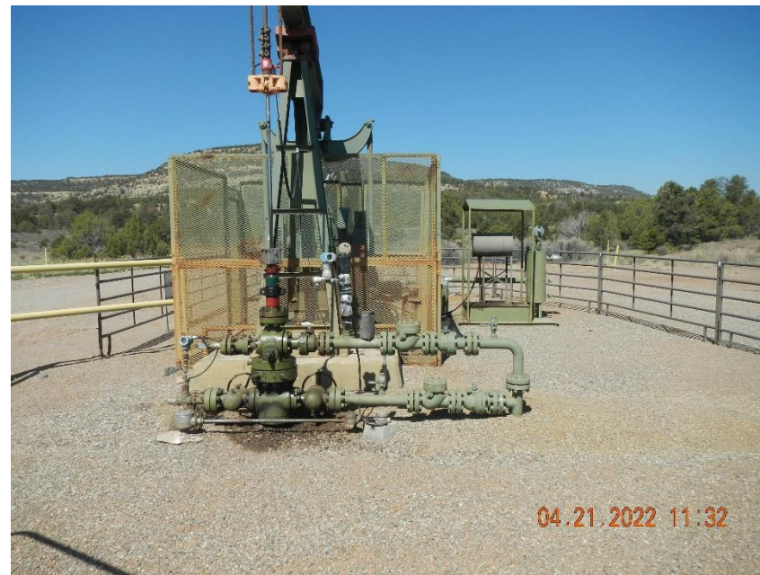
Well head is stained and wet. Surrounding gravel is stained.
