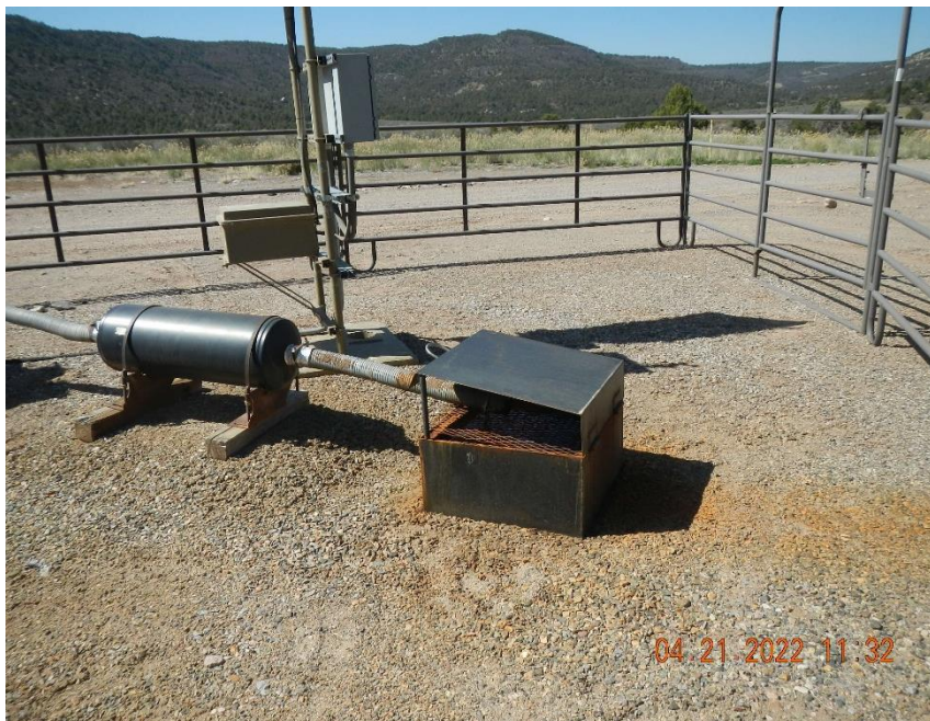
Containment for prime mover exhaust is almost full of fluids.
