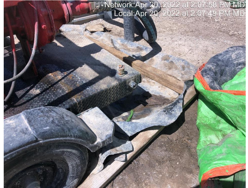
Photo #5611 Insufficient secondary containment and potentially impacted soil under tarp.
