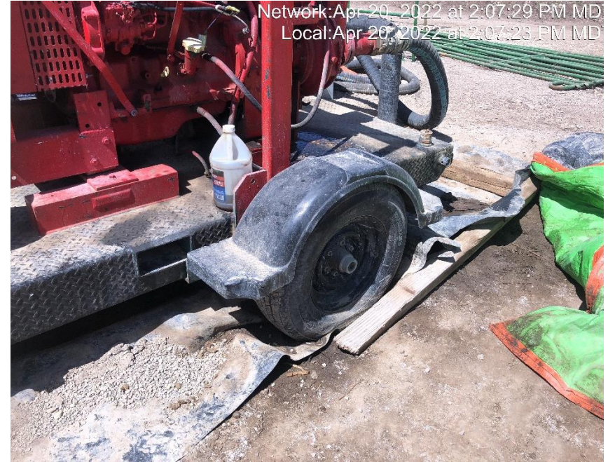
Photo #6509 Insufficient spill prevention BMP.
