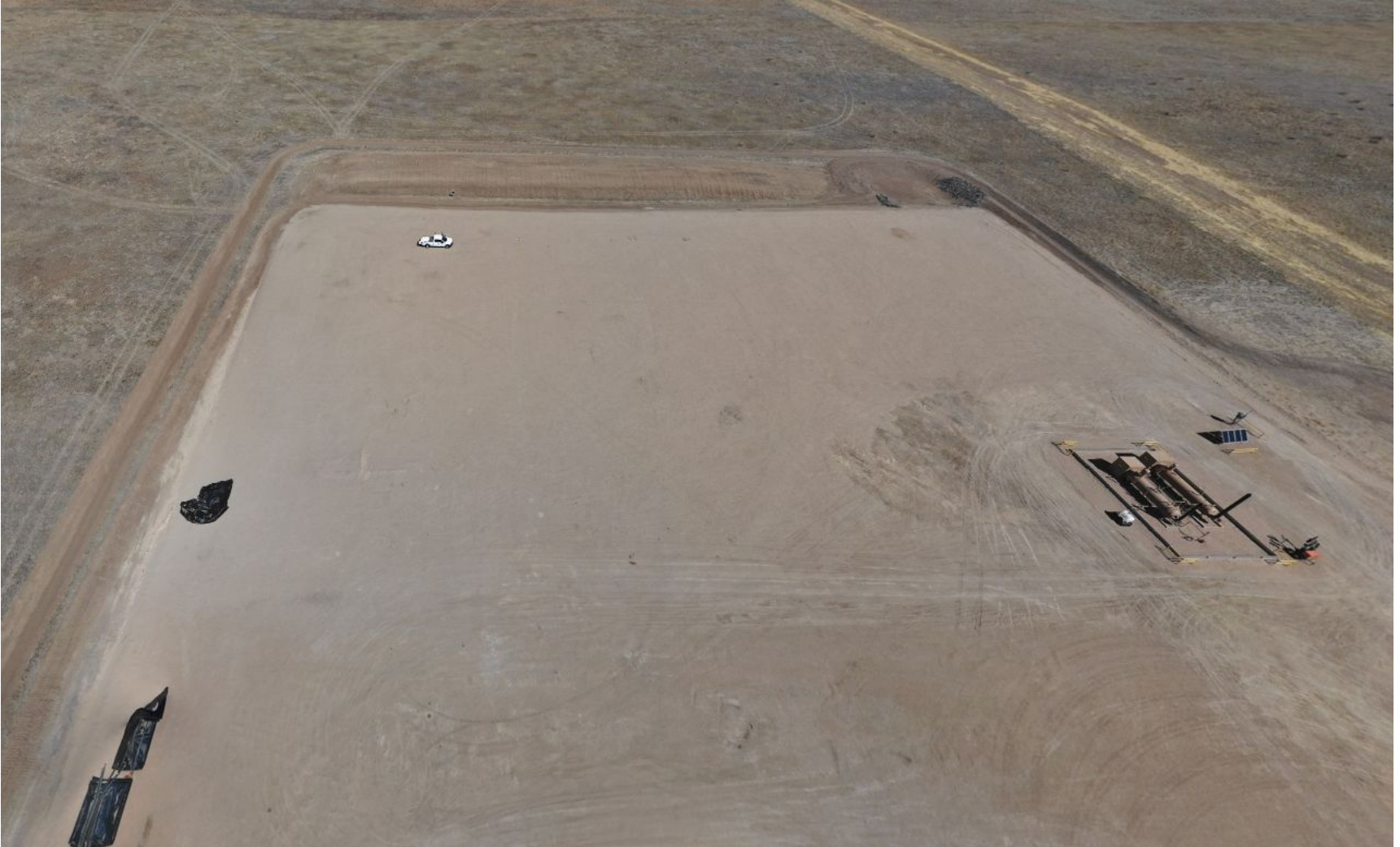
Photo 1. Drone aerial imagery illustrates the northern Castor location. Photo illustrates the Operator has stabilized the location was roadbase.
