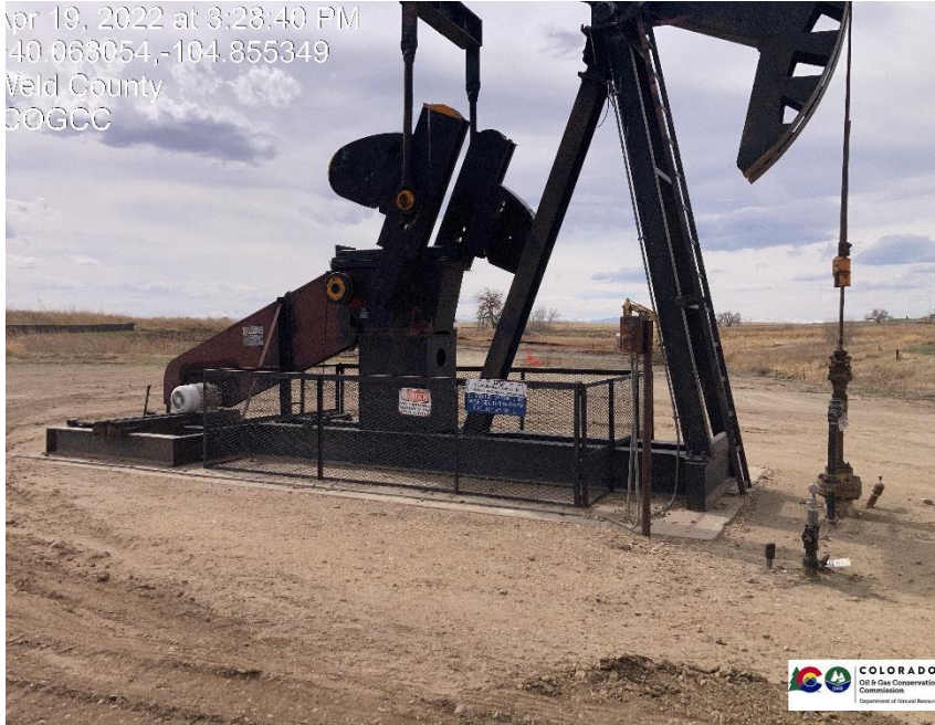
Pic 1 wellhead / pump jack
