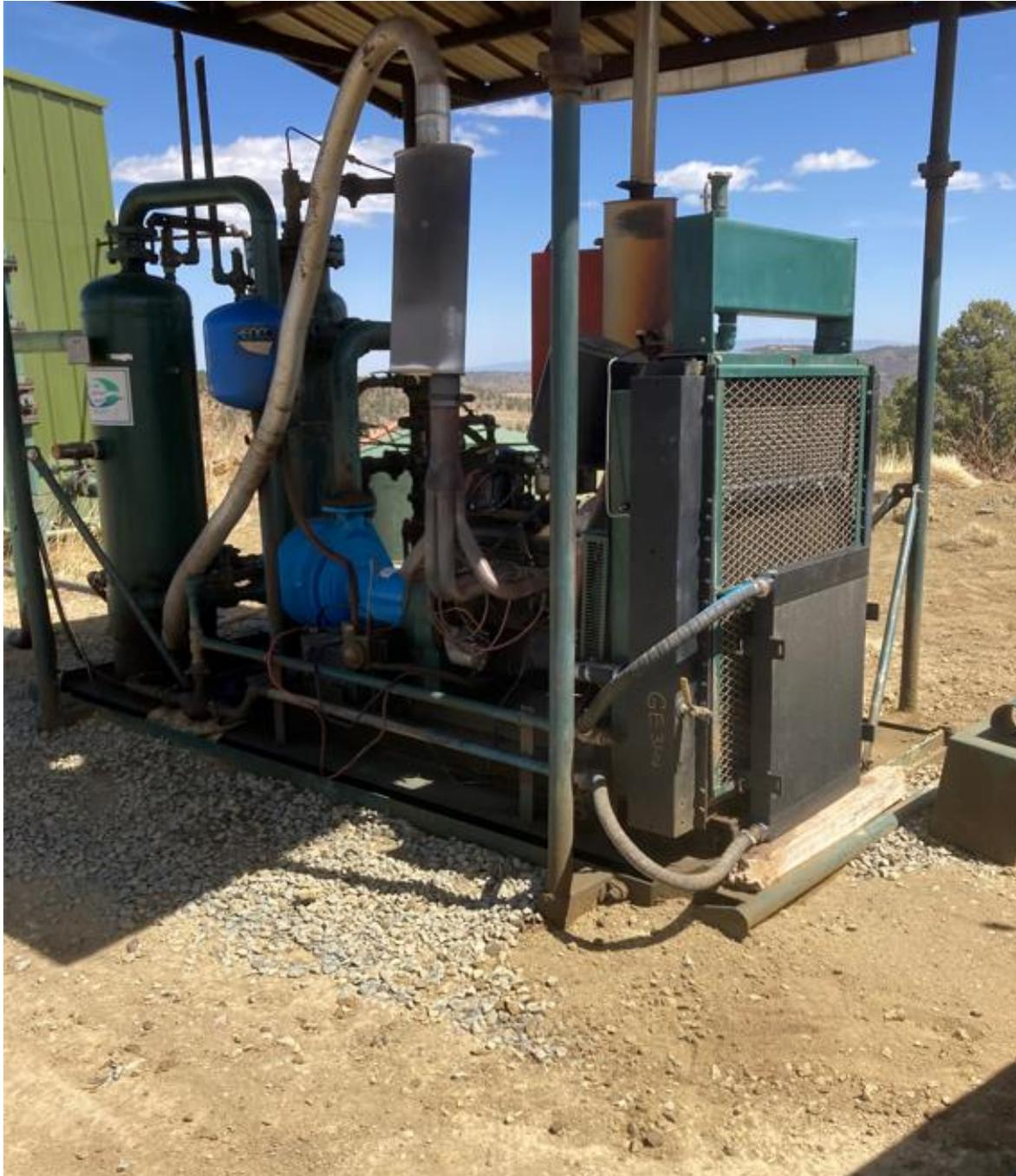
PHOTO 1: EQUIPMENT MAINTENANCE HAS BEEN PERFORMED, THE FLUID ACCUMULATION THAT WAS FOUND INSIDE OF THE CONTAINMENT SKID OF THE LIQUID RING COMPRESSOR WAS REMOVED. THE IMPACTED SOIL NEAR THE LIQUID RING SKID WAS REMOVED AND THE SELF INSPECTION PROCESS HAS BEEN REVIEWED. CORRECTIVE ACTIONS COMPLETED 4/11/2022.
