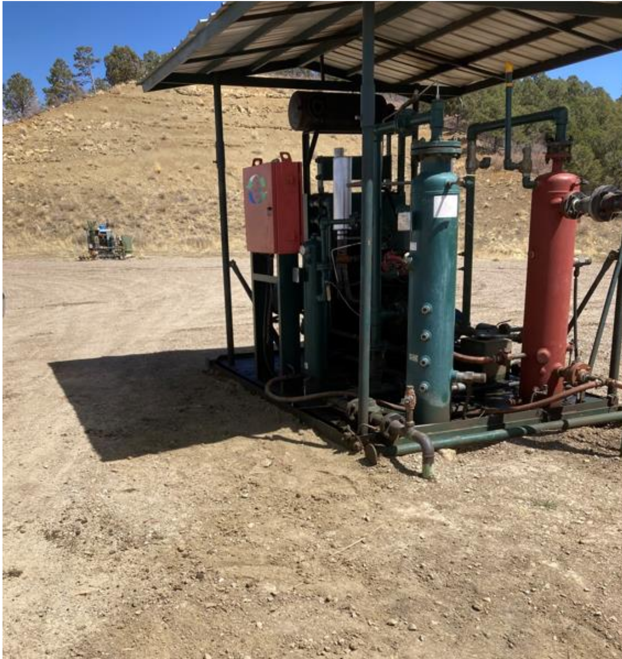
PHOTO 1: EQUIPMENT MAINTENANCE HAS BEEN PERFORMED, THE IMPACTED SOIL NEAR THE LIQUID RING SKID WAS REMOVED AND THE SELF INSPECTION PROCESS HAS BEEN REVIEWED. ALL UNUSED EQUIPMENT WAS REMOVED FROM THE LOCATION AS WELL. CORRECTIVE ACTIONS COMPLETED 4/11/2022.
