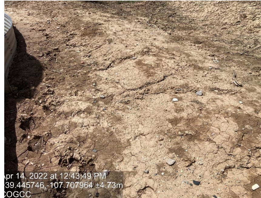
Lack of stabilization/ compaction/ erosion
