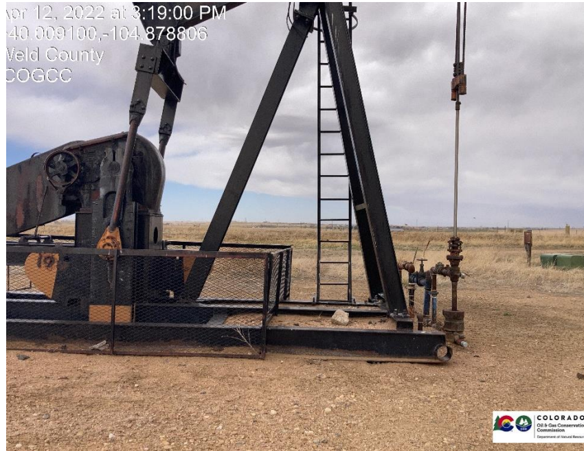
Pic 1 Wellhead, pump jack, electric equipment
