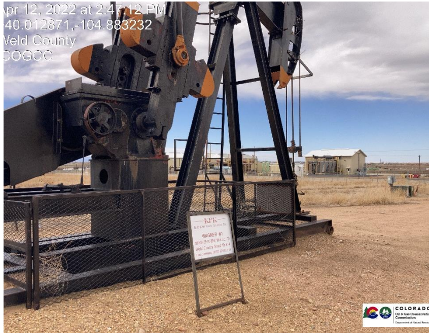
Pic 1 wellhead, pump jack, electric equipment.
