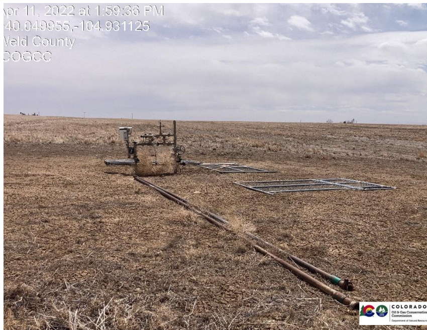
Pic 1 Unused equipment, no wellhead sign posted. Unused equipment needs to be removed.
