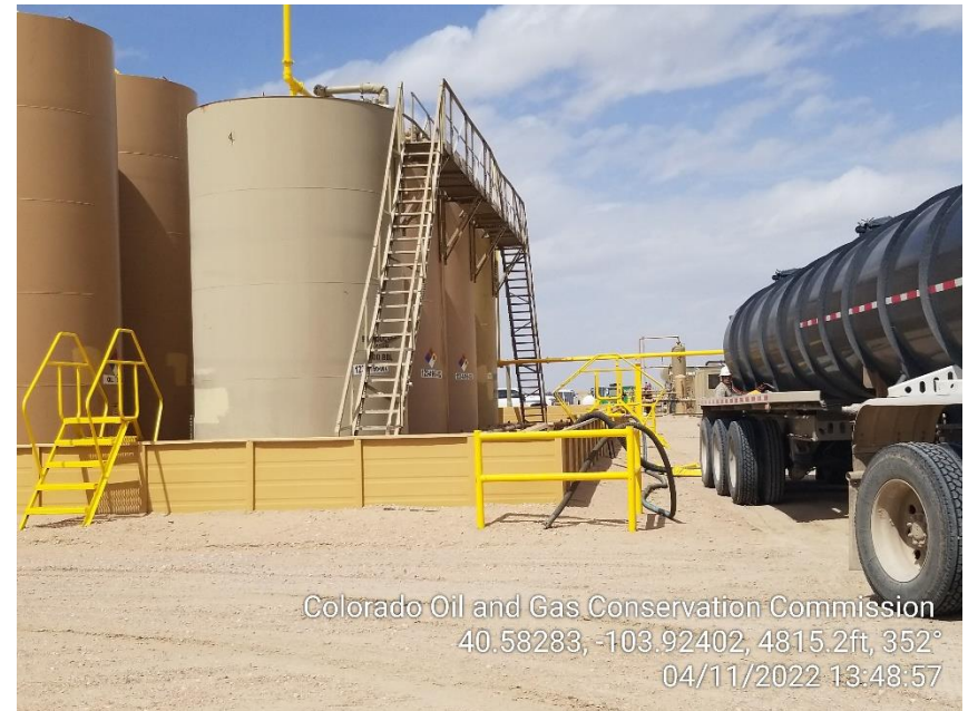
Photo 10 – Tank Battery – Water Tanks
