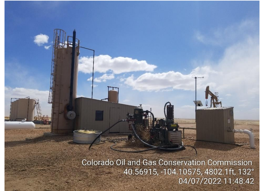
Photo 10 – Heater Treater, Compressor and Gas Meter
