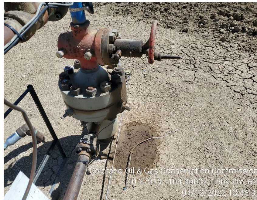
Master valve leak and stained soil
