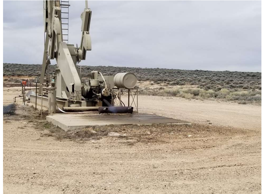
Photo 2. Stained soil at pump jack exhaust.
