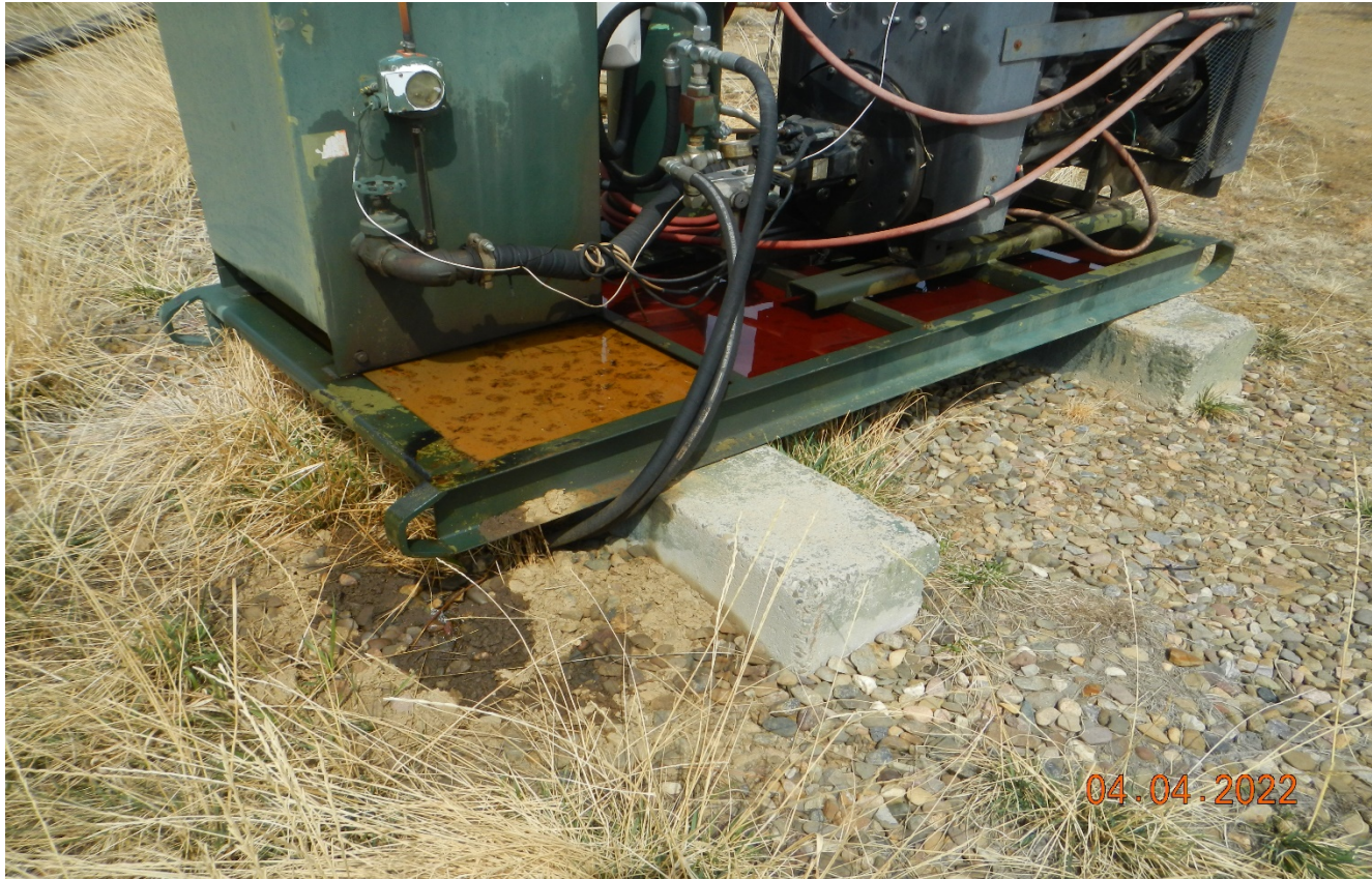
Photo 2. There is oily fluid in the engine skid which is spilling onto the ground.
