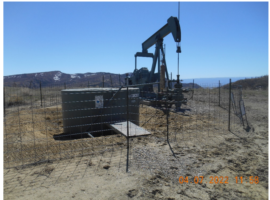
Produce water tank
