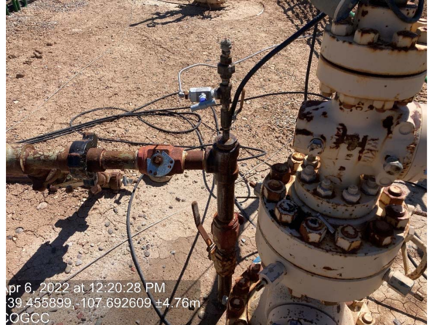
Leaking Braden head line
