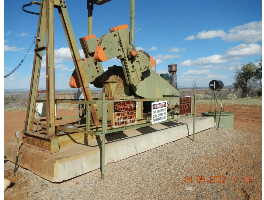
Lube oil container on secondary containment.
