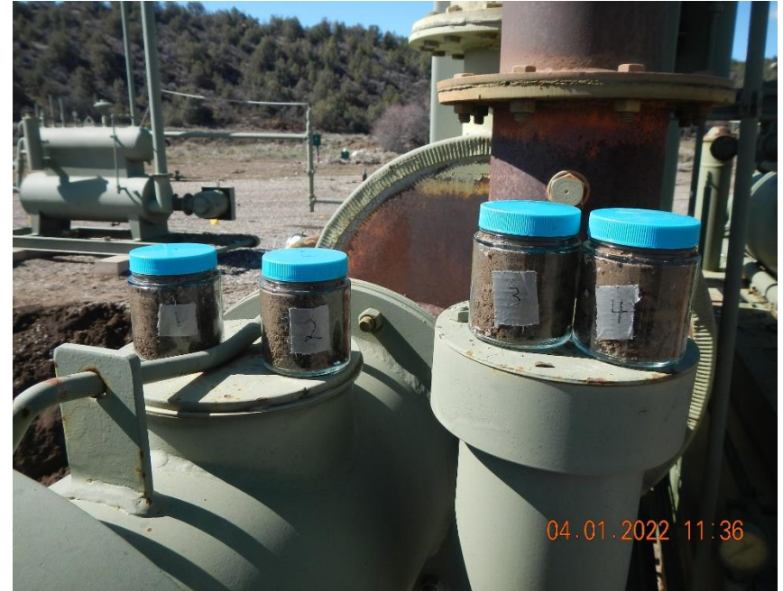
Three discrete samples collected from the west wall and one collected from the base of the excavation.
