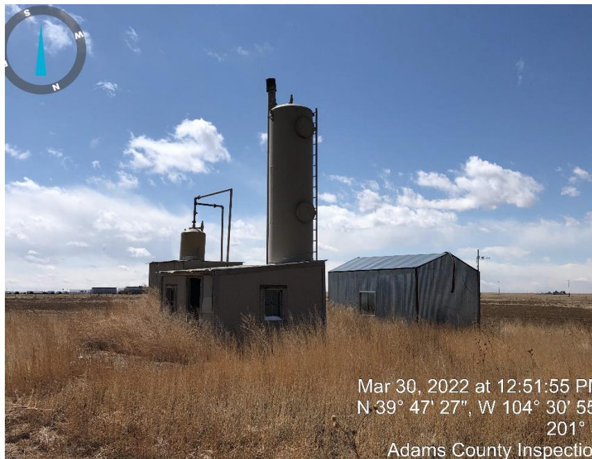
Photo #3 Separator and compressor house.
