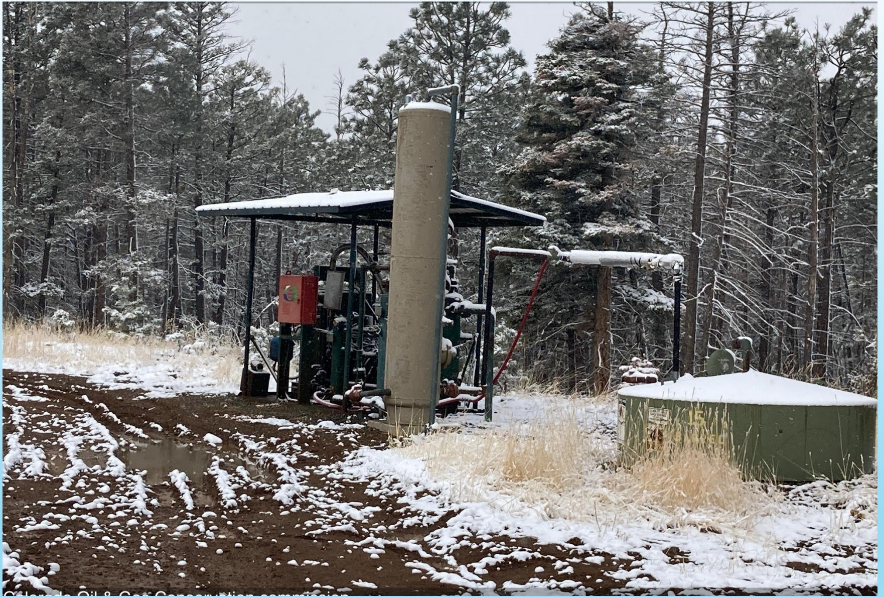
PHOTO 3: WELLHEAD AND EQUIPMENT
