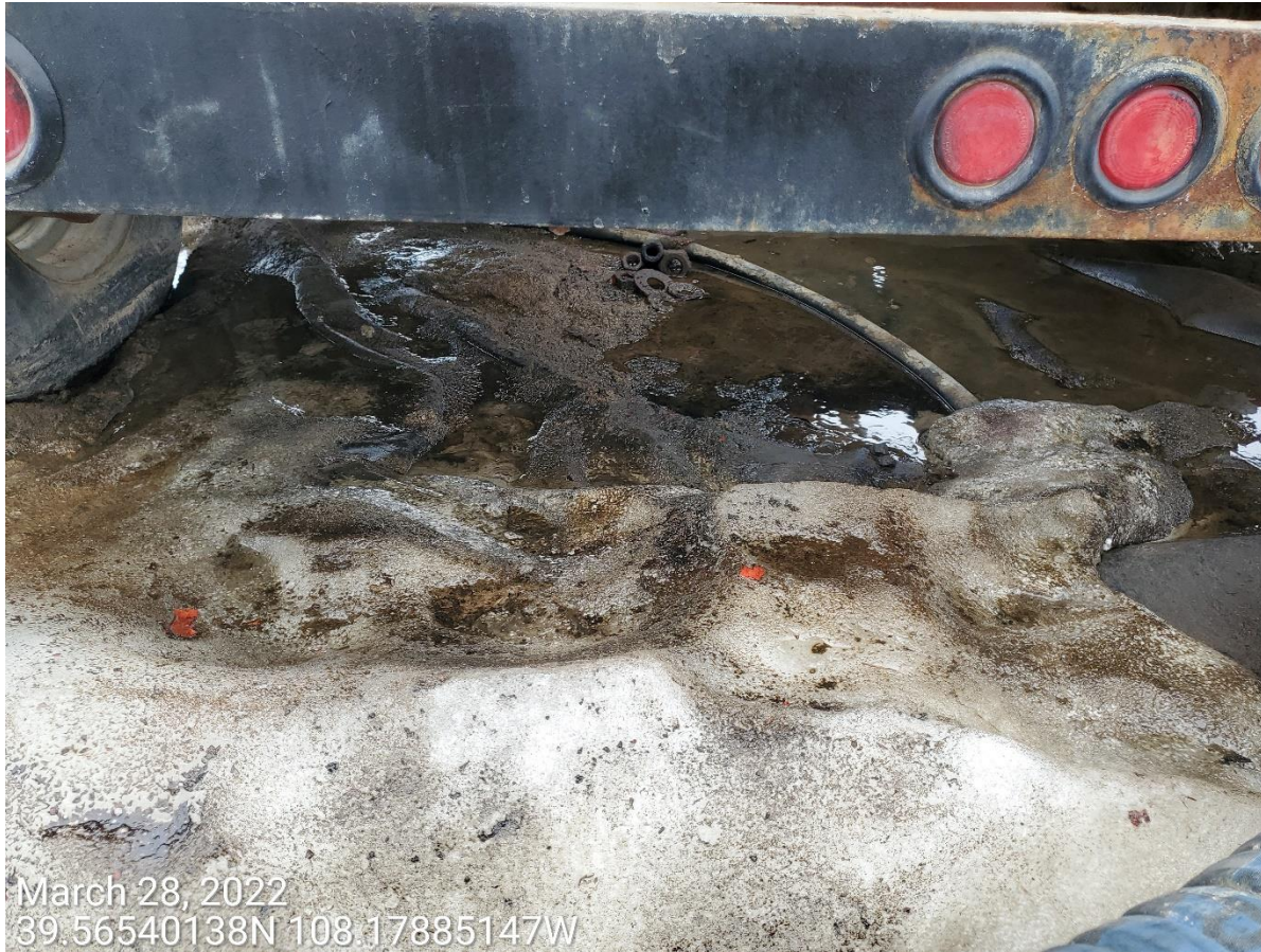
Photo 3: Photo taken from beneath pump trailer. Photo shows leaks/drips and impacting stormwater
