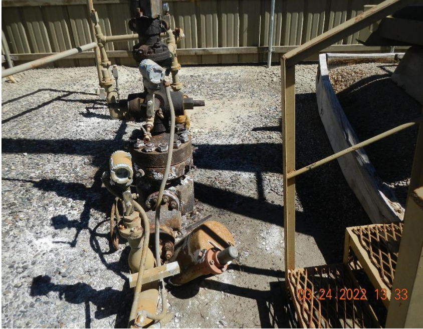
#17-3A well head and surrounding area are stained. Damp soil observed during this inspection.
