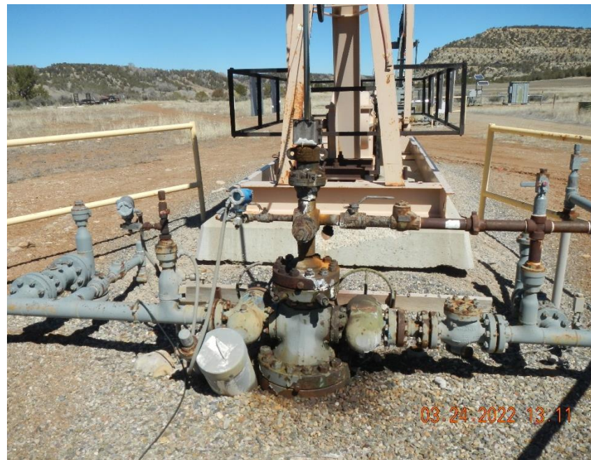
Staining on and around #20-1 well head.
