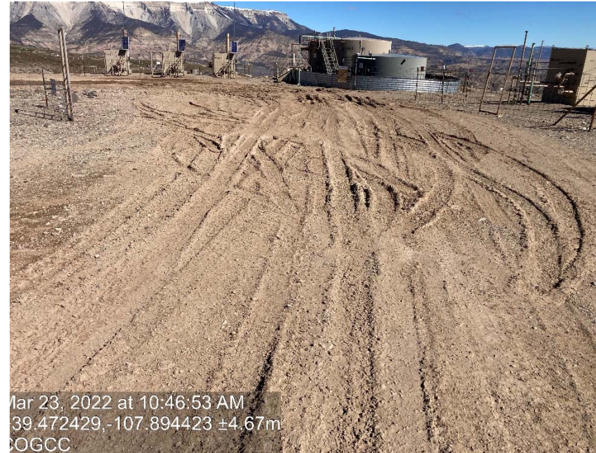
Lack of stabilization/compaction
