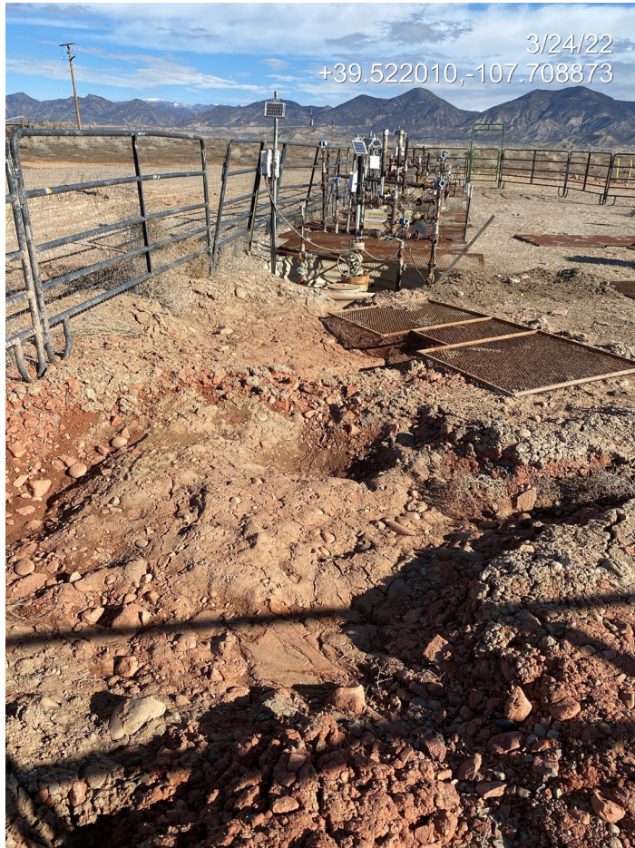
Photo 3. Photo taken from the well area shows unused or improperly installed well cellar grates throughout the well area.
