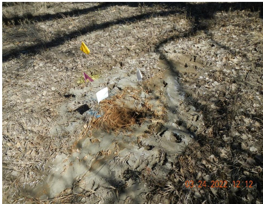
Area where Spill/Release Point ID #481824 day lighted. An approximately 1' diameter hole was observed.
