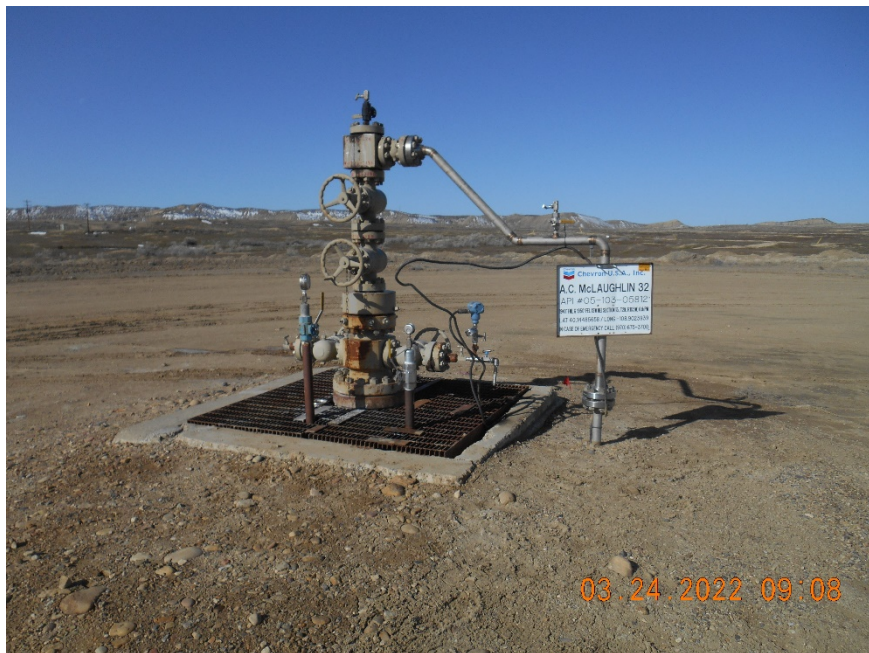
Injection wellhead
