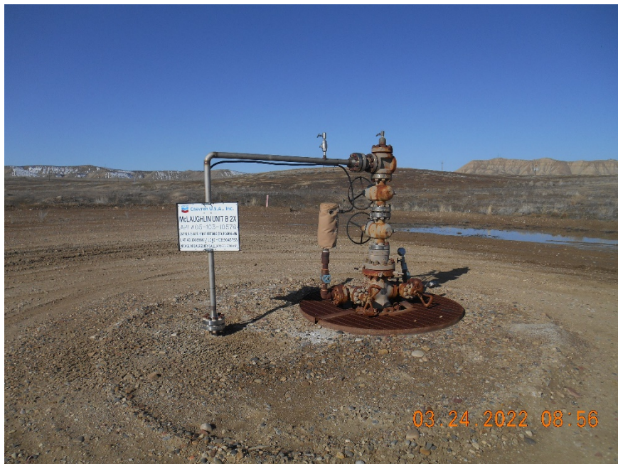
Injection wellhead
