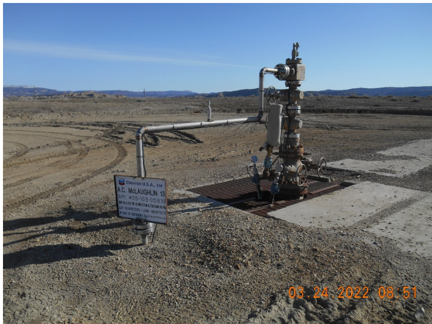
Injection wellhead
