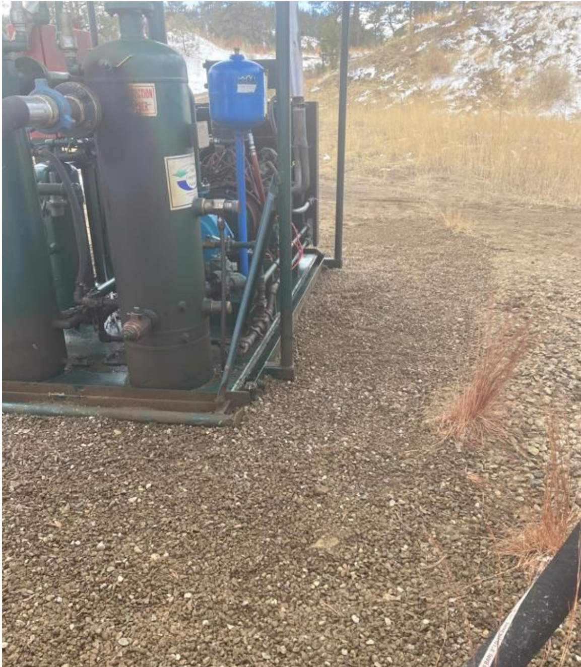
PHOTO 1: MAINTENANCE HAS BEEN PERFORMED, THE IMPACTED SOIL NEAR THE ENGINE SKID WAS CLEANED UP AND REMOVED FROM LOCATION.
