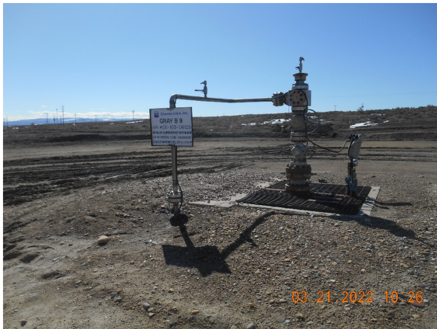
Injection wellhead
