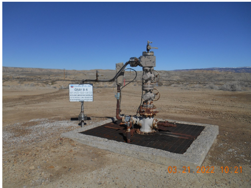
Injection wellhead
